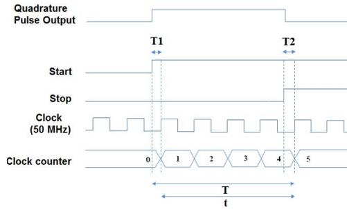
Fig. 4. A-method timing diagram
